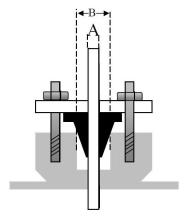
1. To replace a faulty gland packing with a valve cone the dimensions of the valve must be supplied.
